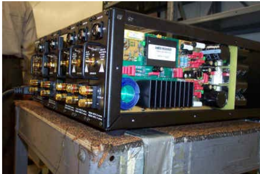
One of the first of ARC's new 150M amplifiers to come off the production line. It uses a new digital switching "class T" output stage.
